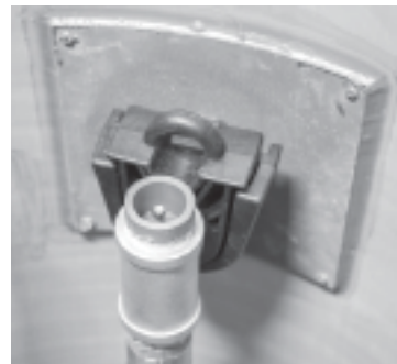
Make a smooth, continuous fillet around the seam between the mounting plate and riser.
