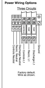
Installations in existing construction may pose issues in providing power to the septic panel. A suggestion is to install a sub panel, like they do for a hot tub instattation.
