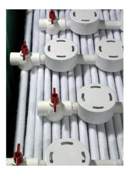
Inspect the interior of the pod to ensure all the fabric is hanging in the rack. Sometimes they pop out during shipping & installation. It's easy to place them into the grooves.
