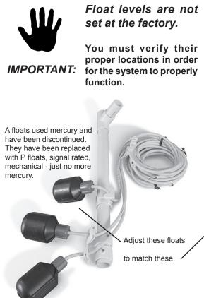
Remove the float assembly from the vault. Loosen the set screw in the upper float holder and slide it to its proper location. The measurement is made from the top of the blue pump vault to the centerline of the cord grip. Retighten the set screw and reinstall the float assembly in the pump vault. *Do not alter the floats' tether lengths.* Make sure the floats can swing freely without hanging up on each other or on the screen so you may need to turn them so they swing free.
