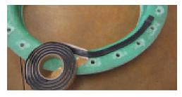
Be sure to place the butyl tape *inside* the bolt holes on the *underside* of the flange.
