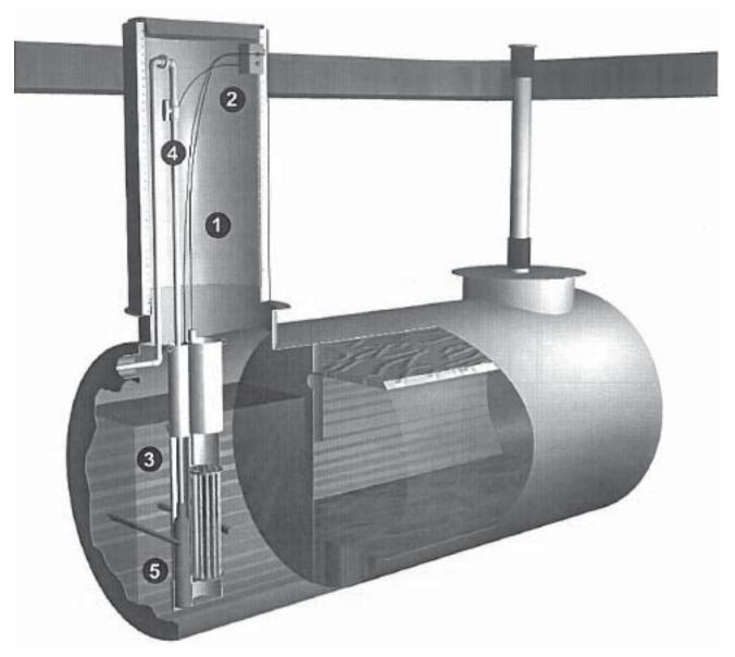
The Anchorage Tank & Welding, Inc. S.T.E.P. System is a combination of a specially designed Anchorage Tank septic tank and Orenco Systems<sup>®</sup>, Inc. riser, pumps, and controls.
