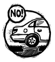
**DON'T** drive over your tank or any buried components in your system, unless it's been equipped with a special traffic lid. If the system is subject to possible traffic, put up a barricade or a row of shrubs.
