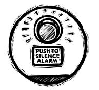
**DO** remember that the audible alarm can be silenced by pushing the lighted button located directly above the "Push to Silence" label on the front of the electrical control panel. With normal use, the tank has a reserve storage capacity good for 24-48 hours.
