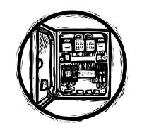
**DO** locate your electrical control panel where it will be protected from potential vandalism and have unobstructed access.
